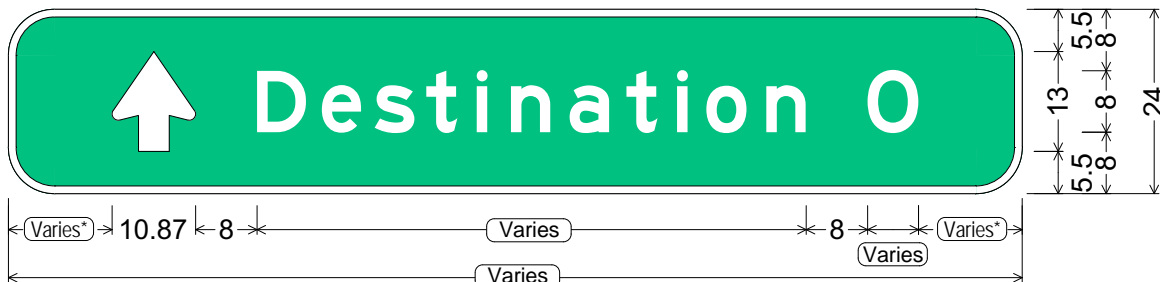
D1-1a (ramp - crossroad); 6.00" Radius, 1.00" Border, White on Green; Arrow 8" Type D1 - 90°; "Destination" E; "0" E;
