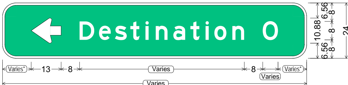
D1-1a (ramp - crossroad); 6.00" Radius, 1.00" Border, White on Green; Arrow 8" Type D1 - 180°; "Destination" E; "0" E;
