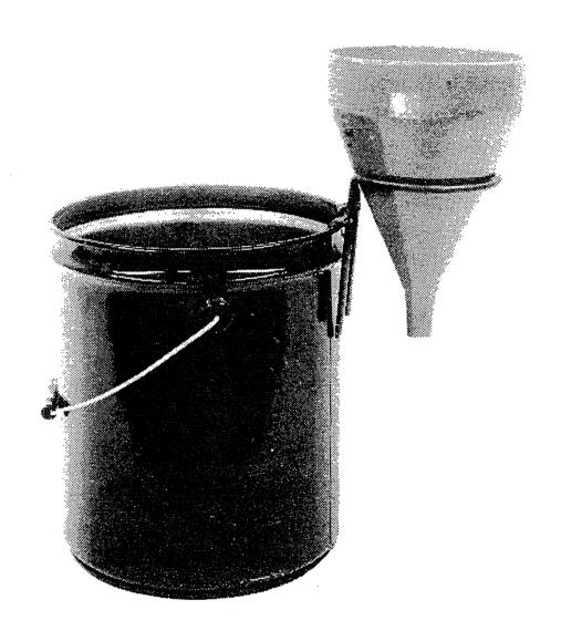
Grout Flow Test Apparatus
