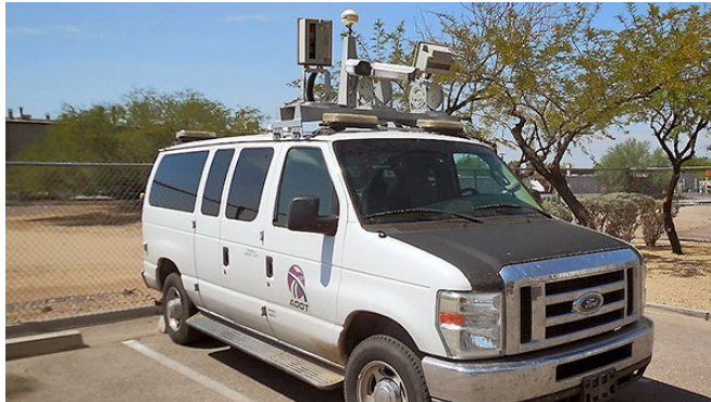
This photolog van was used by ADOT in 2013. It was outfitted with high-definition cameras and lasers mounted on top of the van.
