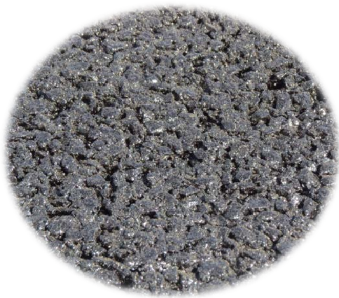
AR-ACFC Rating Excellent Pavement
