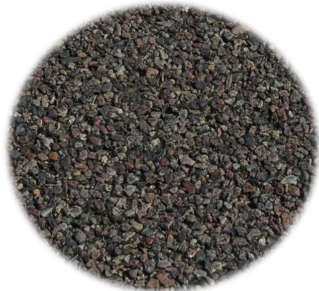
AR-ACFC Rating Unacceptable Pavement
