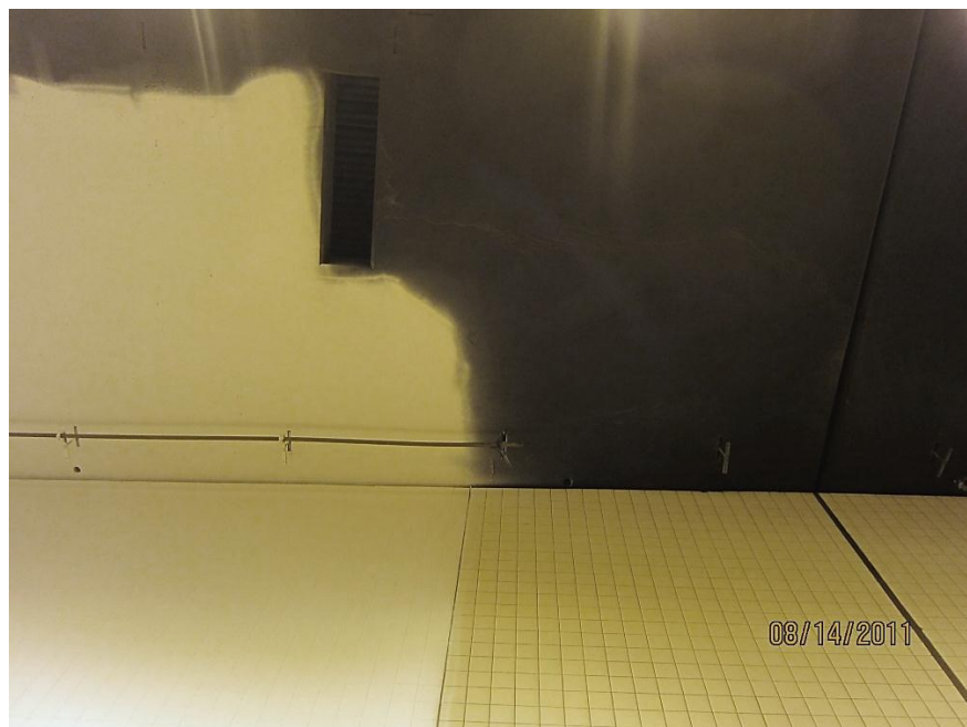
Photo of the Test Area inside the eastbound threshold that demonstrates the extreme difference between the reflectance of the new white coating and that of the existing dark ceiling surface
