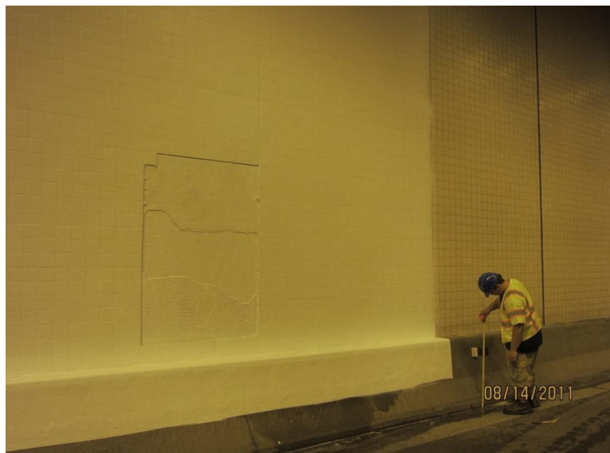
Test Area inside the eastbound threshold where the white coating has been applied to the 30” high concrete “curb”
