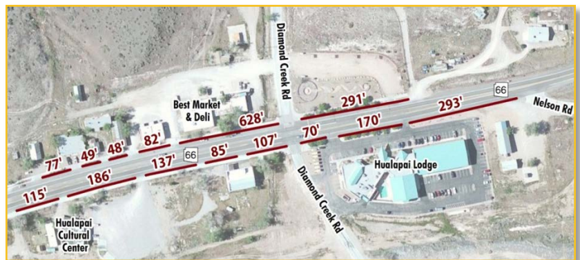
Approximate driveway spacing on SR 66 in Peach Springs.
