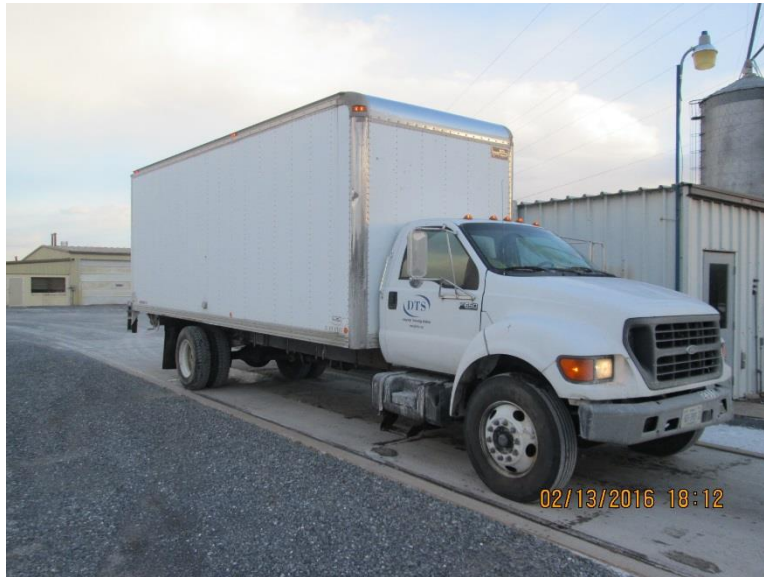
Photo 5-2 – Class 5 WIM Calibration Test Truck
