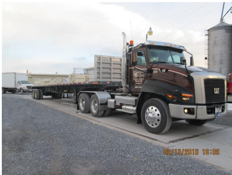
Photo 5-1 – Class 9 WIM Calibration Test Truck
