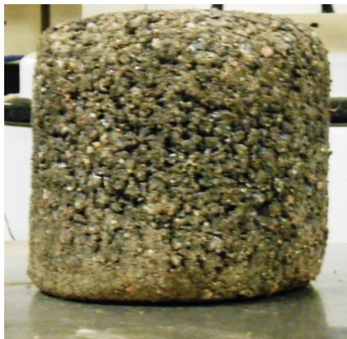
Figure 3. Unaged Cantabro Specimen after Testing
