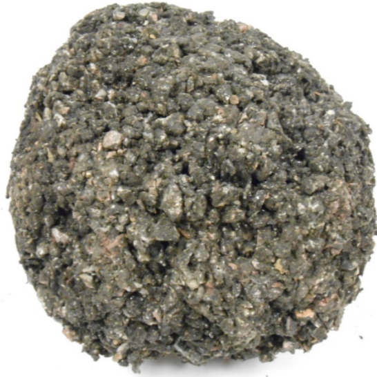
Figure 4. Aged Cantabro Specimen after Testing
