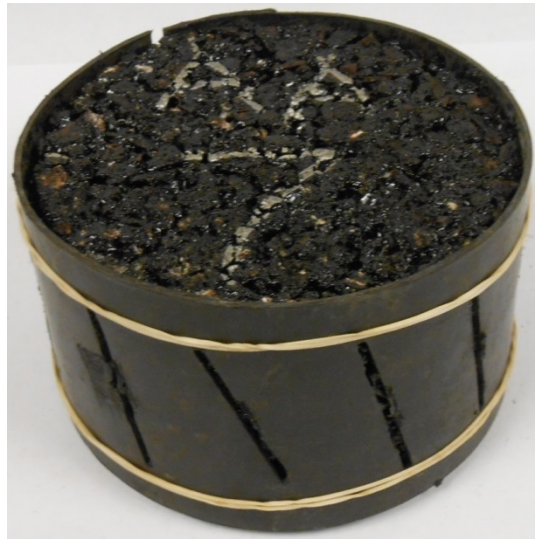
Figure 6. Test Sample after Sample Is Placed in Sleeve
