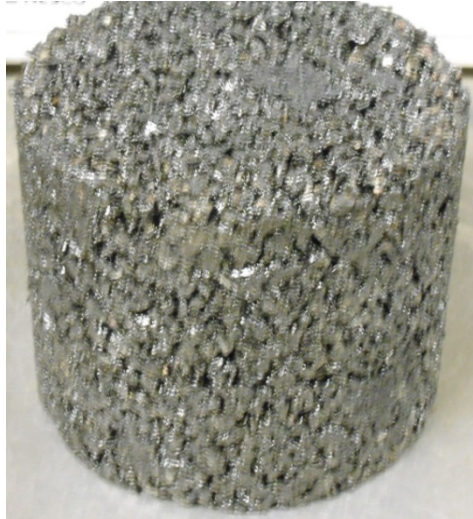
Figure 2. Unaged Cantabro Specimen as Manufactured Prior to Testing
