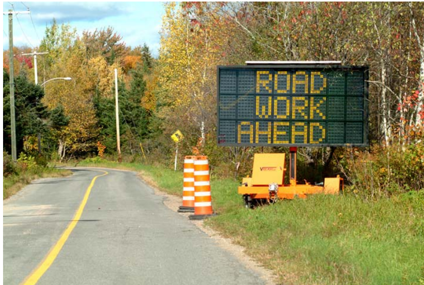
Figure 3. Portable CMS. (Photo courtesy of Ver-Mac, Quebec, Canada)
