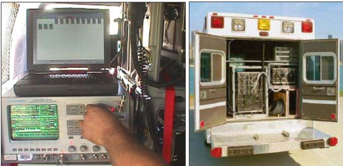
Figure 12 – Typical ACU-1000 System Configuration for Mobile Operations
