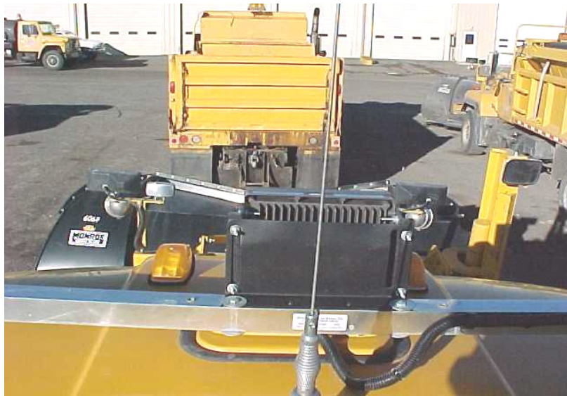
Figure 13. Radar Antenna on Bar: View of Roadway Over Snowplow Blade
