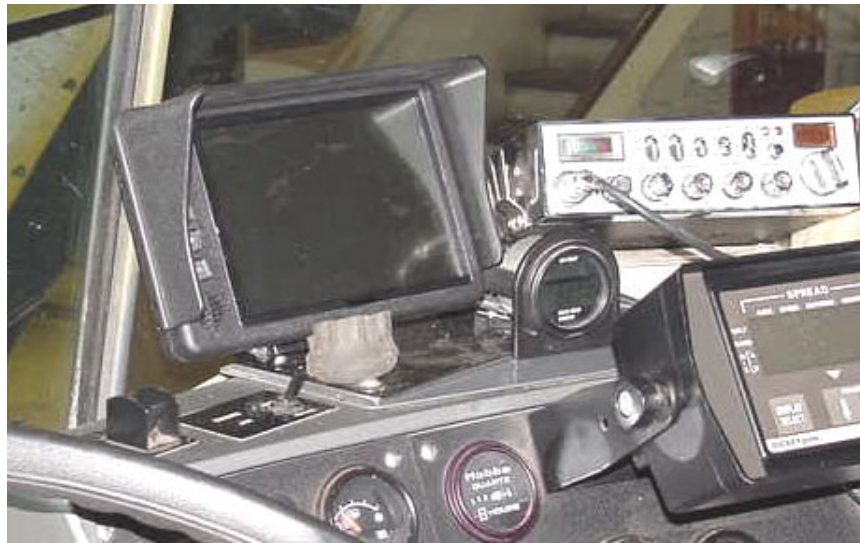
Figure 17. Bendix Upgraded Flat Screen LCD Display: Dashboard Mounting
