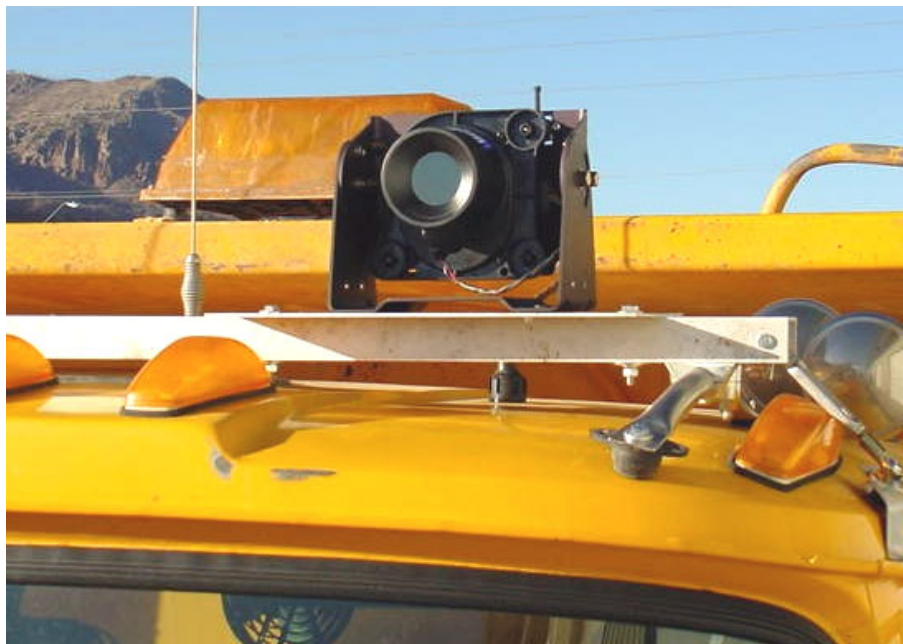
Figure 15. Original XVision Camera Installation on Snowplow F235
