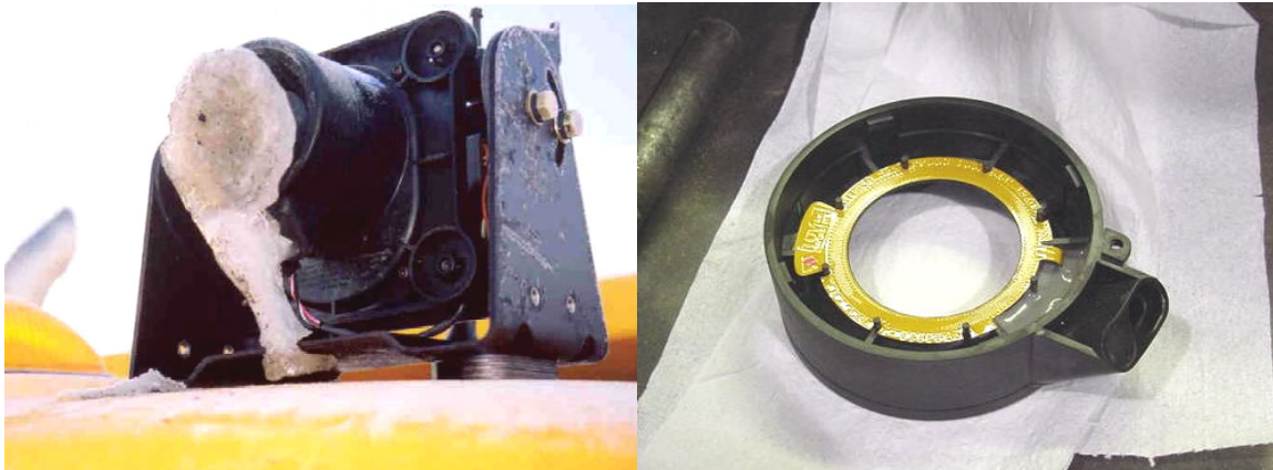
Figure 24. Freeze, Thaw, and Refreeze: the Camera Window Heating Element
