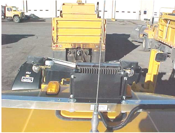
Figure 15: Eaton VORAD Radar Antenna Installed on ADOT Plow
