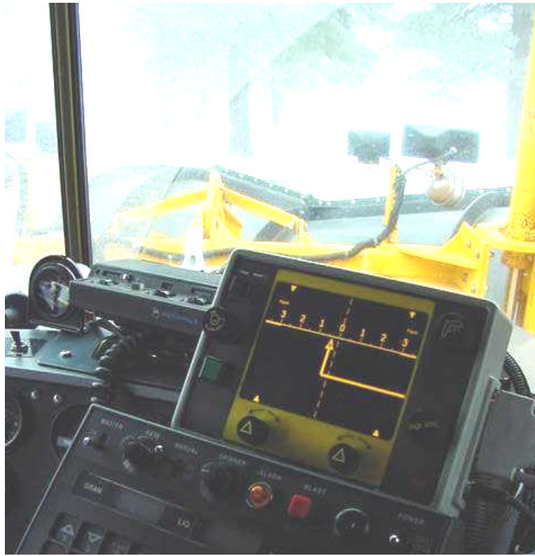
Figure 11: 3M Operator Display Screen in ADOT Plow F342
