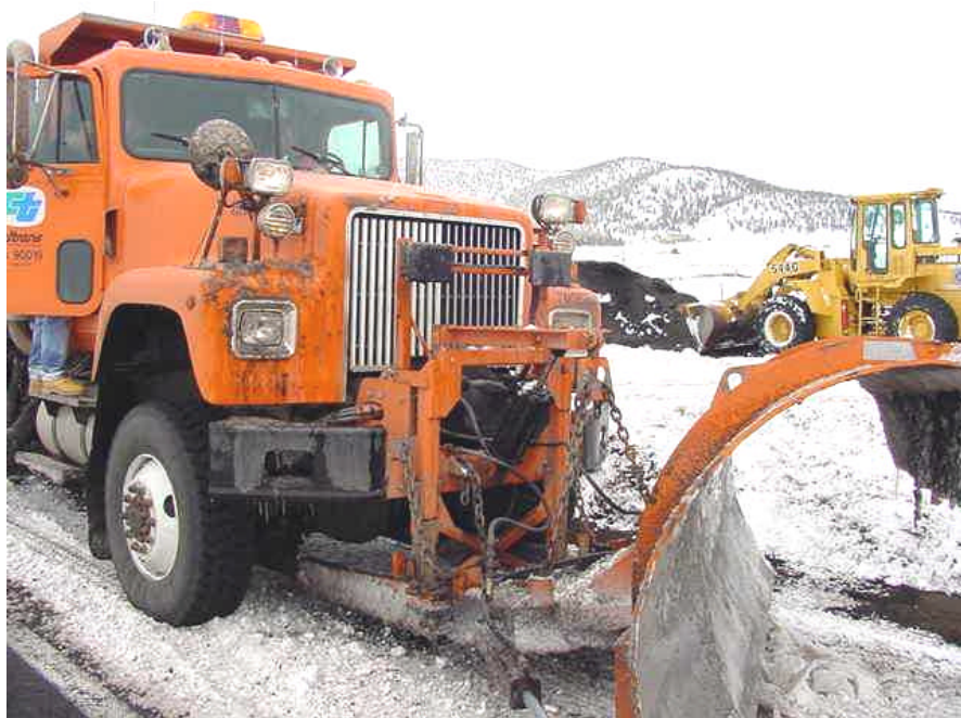
Figure 18: Loading Cinders During Plowing Operations – Kendrick Park
