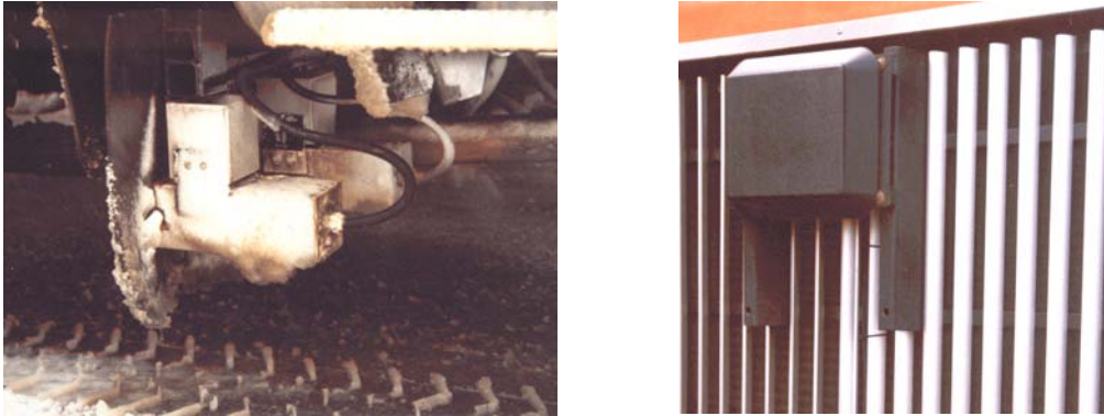
Figure 30: ASP-I - Magnetometers (L) and CWS Radar Antenna
