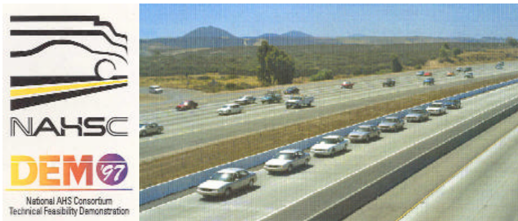
Figure 2: Demo '97 - Platoon Testing near San Diego on I-15 [photo by PATH]
