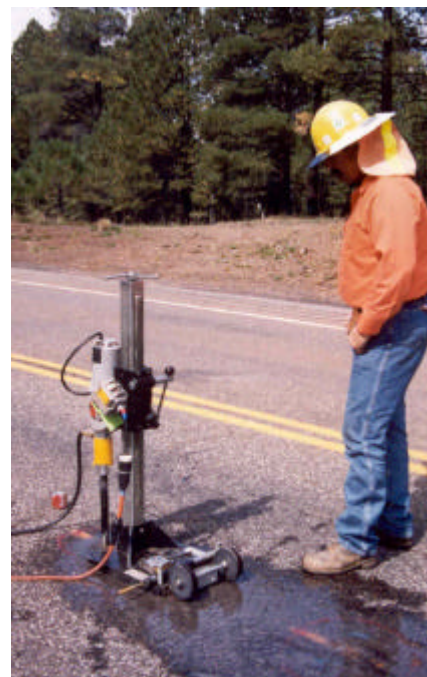
Figure 23: Caltrans Pneumatic Percussion Drill (L) and ADOT Electric Core Drill
