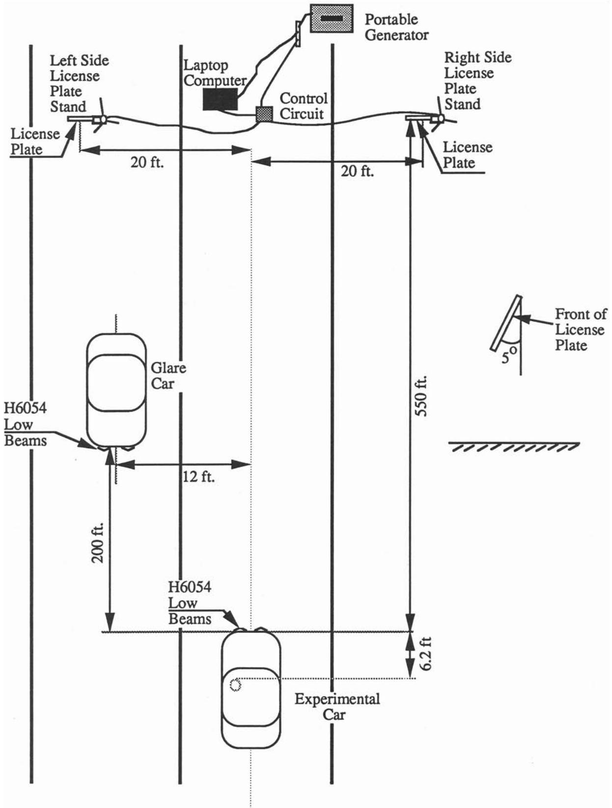
Figure 2. Setup for Nighttime Conspicuity Experiment
