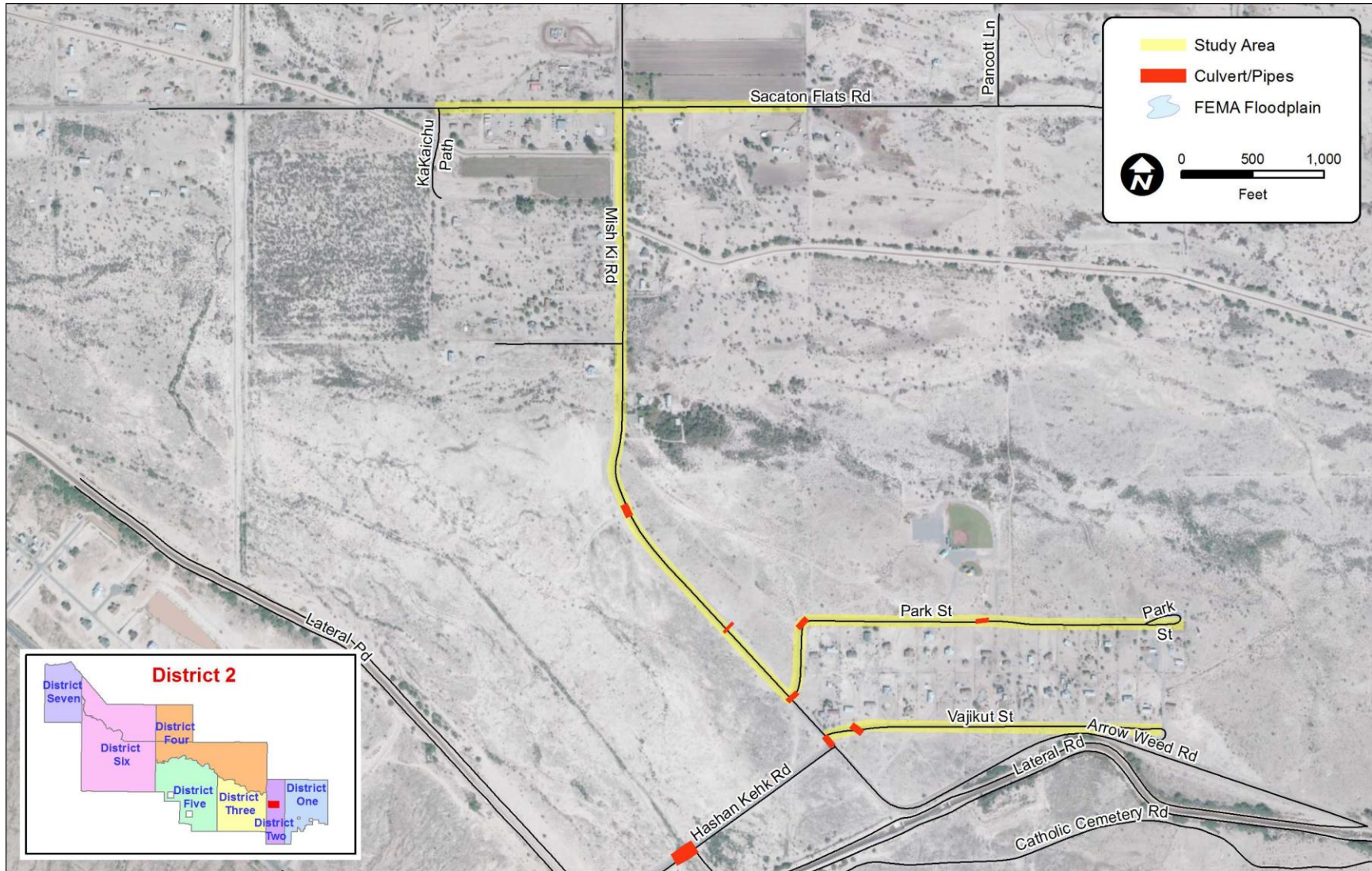
Figure 2-5: District 2 Drainage Infrastructure
